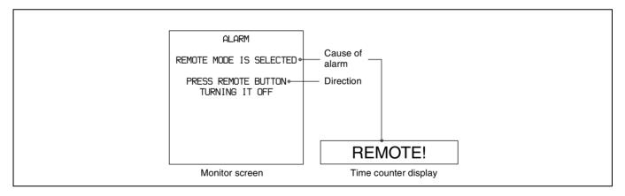
If such an alarm message appears, a connection or operation error may have been made, or condensation on heads may have occurred. Follow the direction indicated on the monitor screen.
